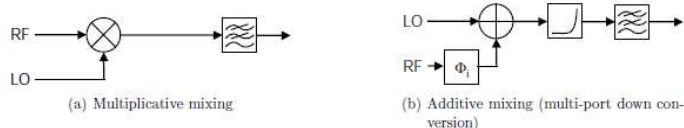
Fig. 1: Multiplicative versus additive mixing. The additive mixing process is the basis of the multi-port theory
