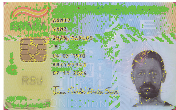
Fig. 7. Ideal document template (from MIDV-500). Yellow points represent the keypoints in variable data zones, which are not used for document location and identification. Green points represent static element keypoints, their neighborhoods are used for descriptors computation
