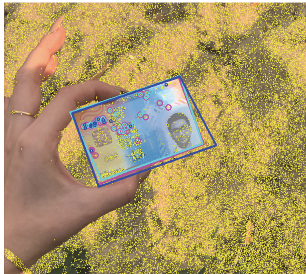
Fig. 8. Analyzed image (photo esp_id/44). Yellow points represent all detected keypoints. Document location results and keypoint inliers are shown in color (SURF — blue, BEBLID-256 — cyan, BEBLID-512 — magenta)
