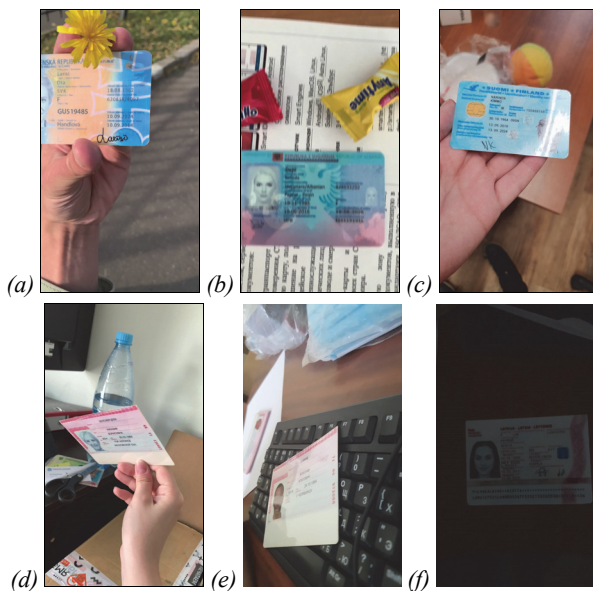
Fig. 9. Challenging conditions for capturing the identity documents, as shown in MIDV-2020 dataset: a) partial face (frame svk_id/66/000145); b) defocus (frame alb_id/55/000019); c) reflection (frame fin_id/90/000253); d) shift in space (frame rus_internalpassport/87/000301); e) unconstrained shooting angle (frame rus_internalpassport/70/000133); and f) bad illumination (frame lva_passport/19/000103)
