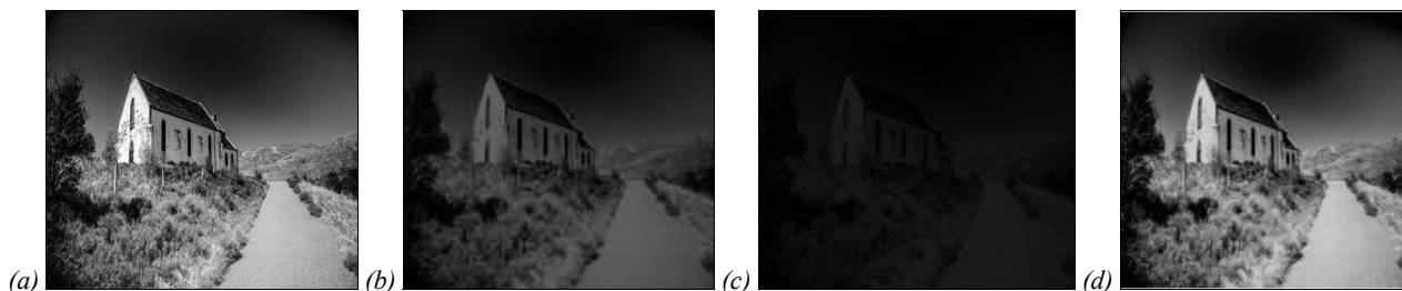
Fig. 4. Improved pseudo-color transformation result 2: (a) Original image, (b) r = 1, g = -1, b = 0.5 , (c) r = -1, g = -0.5, b = 0.8 , (d) r = -1, g = 1, b = 0.5
