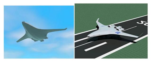
Figure 11.6 – Conceptual project of the eco-friendly quiet passenger aircraft SAX-40
