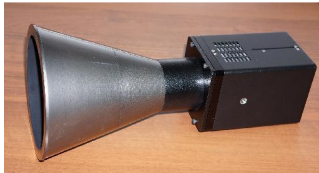
Fig. 4 - Experimental model of star tracker
