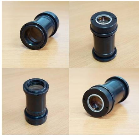
Fig. 2 – Optical system of star tracker experimental model
