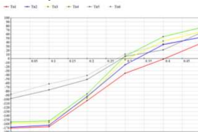
Figure 2 Current-voltage curves of textured samples with p-n junction and coatings of dysprosium fluoride (Tn1, Tn3), erbium fluoride (Tn2, Tn4) and control samples (Tn5, Tn6) without coatings
