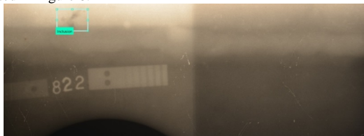
Figure 8. Selection of areas of interest in the form of defects “Inclusion”.
