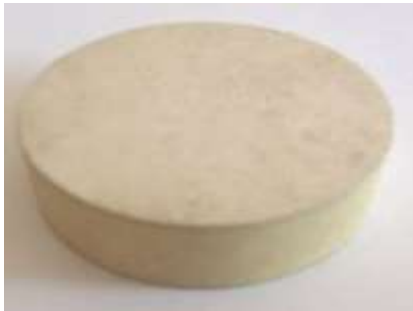
Figure 2. Standard piezoacoustic element with a diameter of 4 mm for a frequency of 1 MHz.
