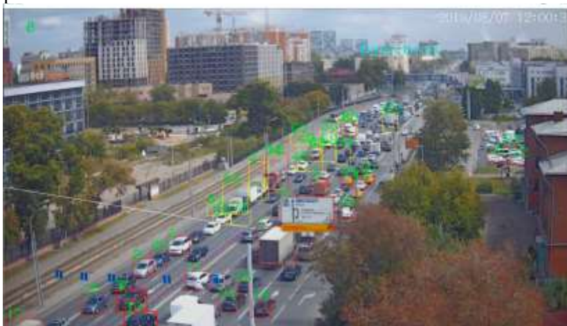
Figure 6. Identified congestion based on vehicle count approach.
