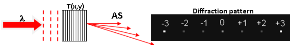
Figure 1. Diffraction on phase grating described by function T(x,y) and imaging of diffraction pattern using AS.
