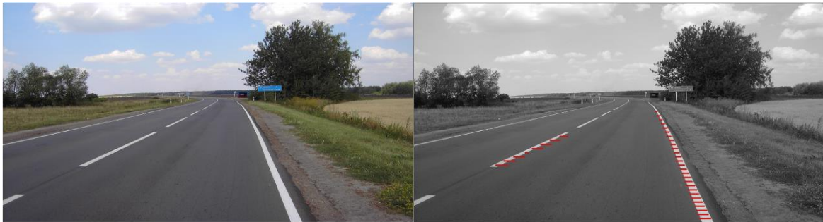
Figure 5. An example of finding a road marking.
